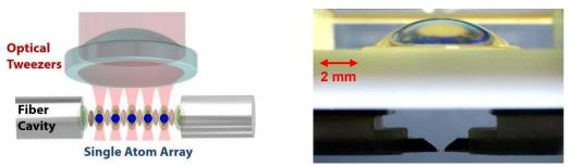
Left: Principle of the experimental setup: An array of optical trap and control a register of single atoms inside an optical micro-cavity. Right: an image of the actual experiment.
